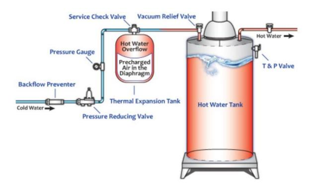
Water expands in volume as its temperature rises. The extra volume caused by thermal expansion must go somewhere. A thermal expansion tank added to your home water system offered the solution to this dilemma.
